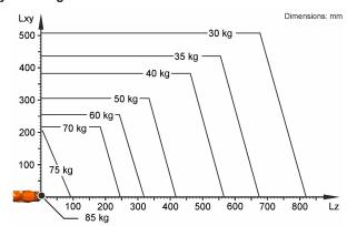
The KR 70 R2100 is designed for a rated payload of 70 kg in order to optimize the dynamic performance of the robot. With reduced load center distances, higher loads up to the maximum payload may be used. The specific load case must be verified using KUKA.Load. For further consultation, please contact KUKA Support.
